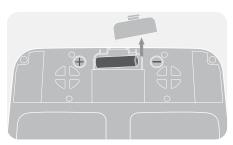
Remove the battery door located on the bottom of the feeder. Insert the (+) positive end of the AA alkaline battery (not included) first, then the (-) negative end into the compartment until it clicks into place. Replace battery door. Your feeder is now on!
